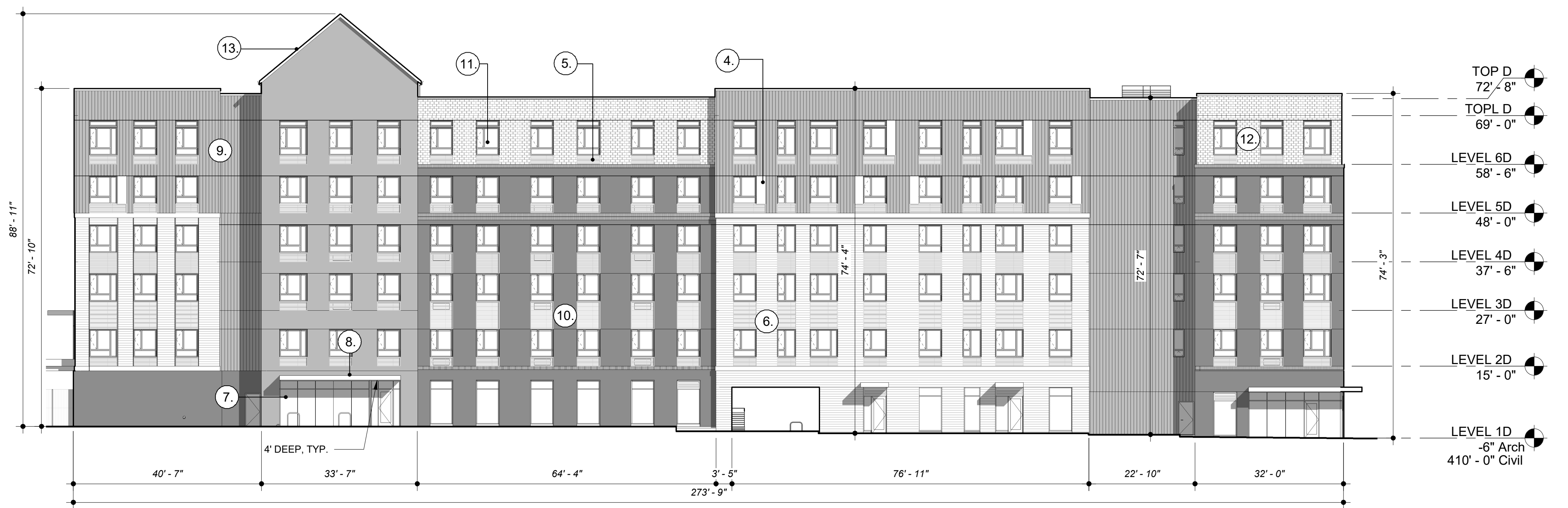
2. DR - BLDG D - NORTH ELEVATION
